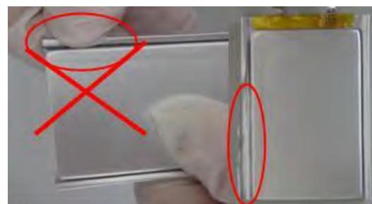
Tabs: The Cell tabs are easy to be broken especially for Aluminum tab. Do not bend the tabs.
