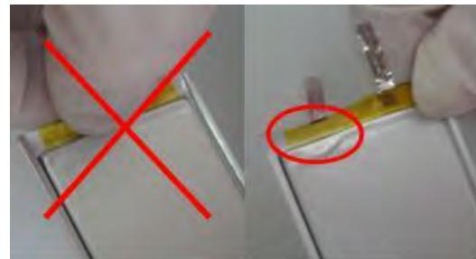
Side Sealing Edge: The side sealing edge has been folded and fixed in cell forming processes and passed hermetic test. The Aluminum foil may brake by re-folding time after time. Don't open and refold this edge.
