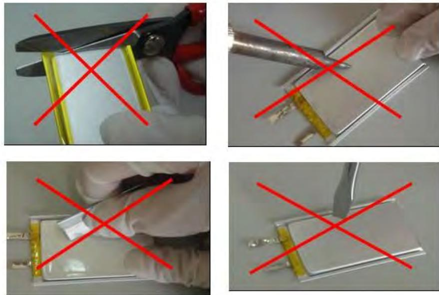
Top Sealing Edge: Sealing edge on the top of the Cell is very flimsy and easy to be delaminated. Do not bend or fold this area.
