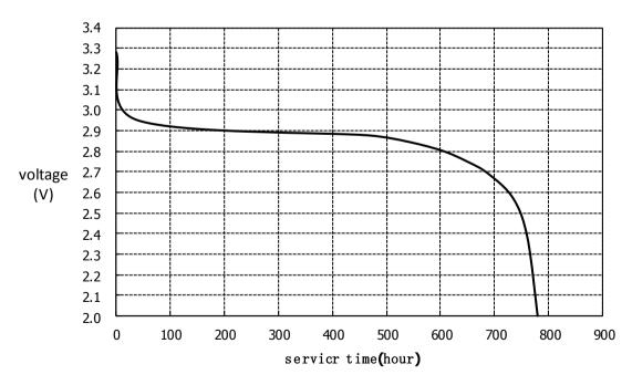
Discharge method:15KΩ, 24 hours/day EV 2.0V temperature of 20±2 $^{\circ}$ C
