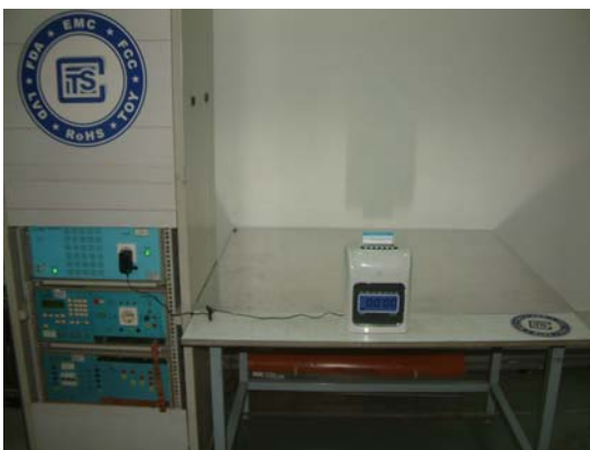
7.3. Photo of harmonic current and flicker emission measurement (H.&F.)
