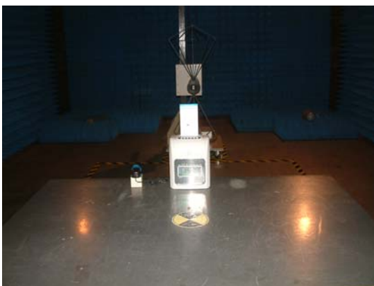
7.2. Photo of radiated emission measurement (R.E. Electric field)
